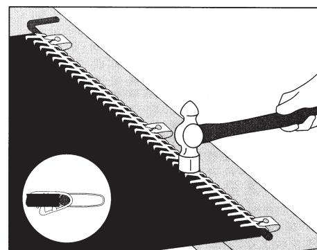
**6.** Hammer lacing completely into top of belt.
