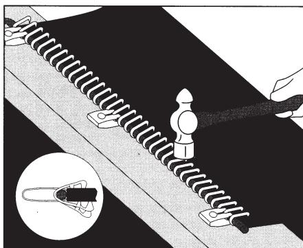
**5.** Turn belt over and hammer lacing halfway into bottom of belt.
