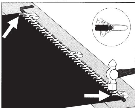
**4.** Using a soft wood surface for support, hammer end teeth halfway into top of belt.
