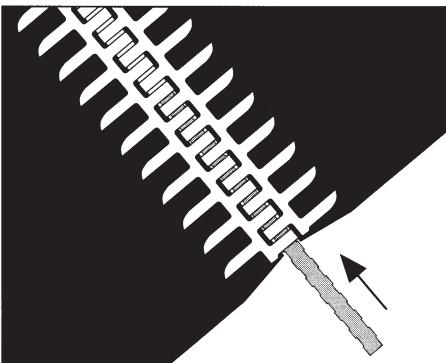
**10.** Repeat steps 1 thru 9 for other end of belt, insert hinge pin and notch belt.
