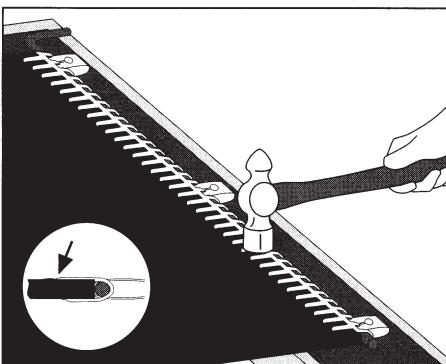
**8.** On hard steel plate, hammer again from top, until teeth are flush with belt surface.
