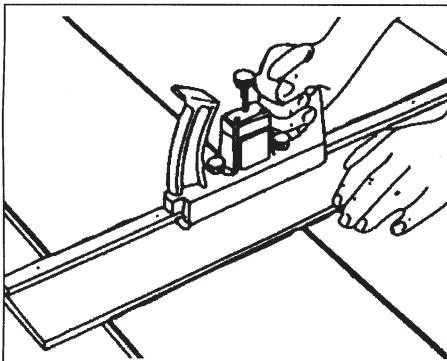
**1.** Square belt ends, then cut using the ALLIGATOR® 300 Series belt cutter.
