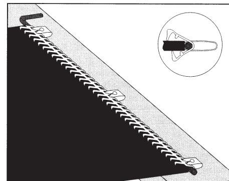
**3.** With bar side up, center lacing on belt holding belt against gauge pin.
