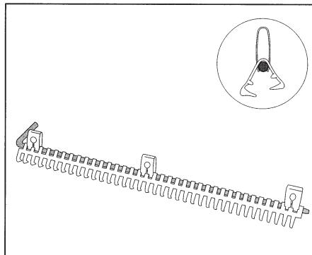
**2.** Place clips on lacing and insert gauge pin.
