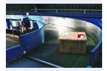
Our curved belts are designed to handle high-speed power turns, saving you time and operational space. What's more, they're also low-noise, for a better working environment.
