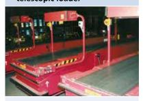
Loading and unloading parcels directly from vehicles with Ammeraal Beltech telescopic conveyor belts simplifies receiving and delivery and it saves time and resources, too. Our telescopic conveyors extend into the vehicle and collapse away after use.
