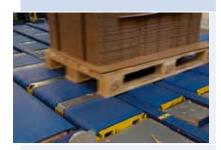
Strength, durability and safety are of paramount concern with floor-level warehouse conveyors, particularly when it may be necessary for employees to step on, off and in between moving
