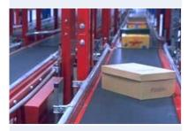
We can offer special profiles and other modifications for increased grip on inclines and declines.
