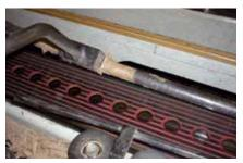
Pletex belts can be hot spliced on site using 'easy to use' QuickSplice tools.
