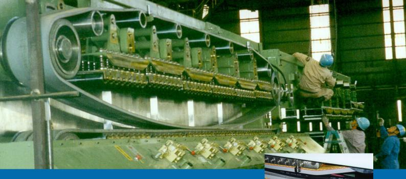
In a number of applications, it is not possible to apply standard Conveyor belting. For example in the cable industry in caterpillars and capstans as cable pulling belts with extreme demands in force/elongation properties. Ammeraal Beltech's endless weaving and coating facilities make it possible to offer a solution made to customer specification for those specific heavy applications.
