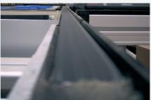
RAPPLON® Flat belts are highly antistatic. It's an essential property when conveying electronic components.
