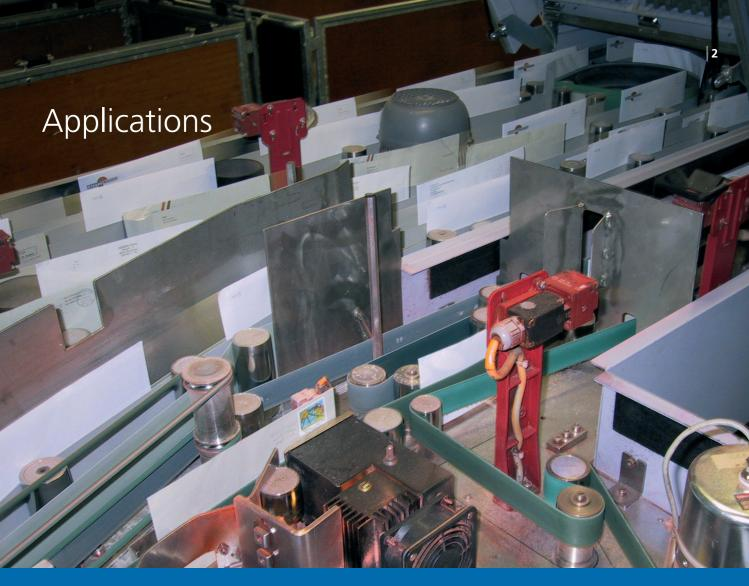
RAPPLON® High performance flat belts serve as drive belts and as machine tapes for industrial processes. Extremely wear-resistant covers, with high grip or low friction, match the ever increasing requirements of uniform and stable speed transmission. To cope with all specific demands our flat belts feature excellent quality coatings like textiles, selected chrome leather, rubber elastomer, natural rubber and thermoplastic elastomers.
