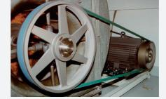
RAPPLON® High performance flat belts perform with an efficiency exceeding 98%.
