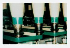
The surface of the RAPPLON® EC-Tape guarantees constant spindle speed although one spindle is braked.
