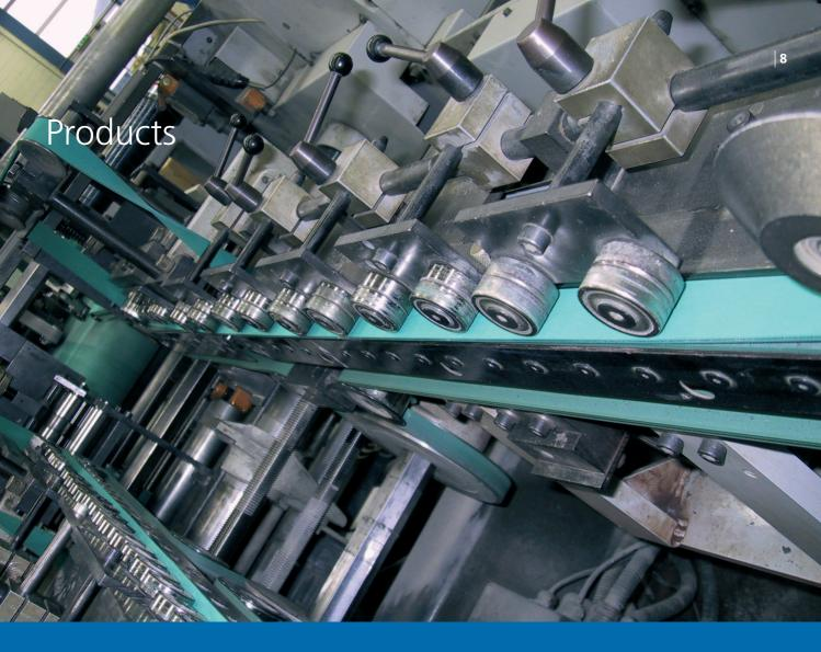
Ammeraal Beltech offers a complete range of traditional polyamide reinforced high-performance flat belt constructions. In addition, we offer belts featuring QuickSplice technology, eliminating the use of adhesives for endless joining.
