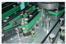
High friction belt covers care for positive conveyance whereas low friction surfaces allow for accumulation and diverting applications in roller drive systems.
