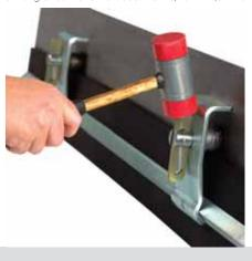
Simply tap loose the locking pin to reposition or replace skirt rubber and then tap to re-lock in place.
